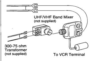
If your TV has both post and plug-type VHF terminals, the post connection is recommended to minimize signal loss.
